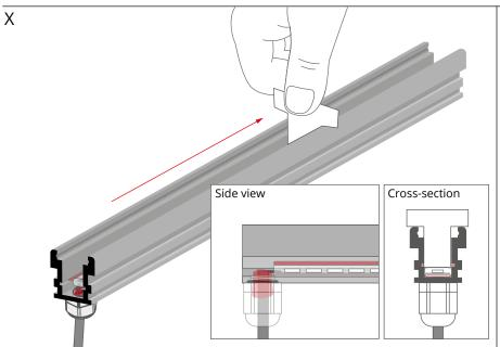
Level the layer of the silicone inside the profile.
