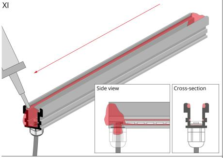
Fill the ends of the profile with silicone.
