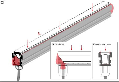
Mount the cover (5) in the profile and press it to the bottom. The excess silicone should come to the surface of the profile and out its ends.
